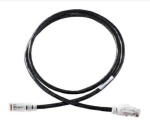
Clarity 6 Modular Patch Cord, black, 15', Category 6, four-pair UTP stranded 24 AWG PVC/CM, center tuned with Clarity 6 connecting hardware for optimum Category 6 installed performance using Ortronics Paralign 2 pair-positioning technology
