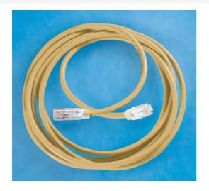
Clarity 6 Modular Patch Cord, yellow, 15', Category 6, four-pair UTP stranded 24 AWG PVC/CM, center tuned with Clarity 6 connecting hardware for optimum Category 6 installed performance using Ortronics Paralign 2 pair-positioning technology
