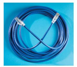
Clarity 6 Modular Patch Cord, blue, 20', Category 6, four-pair UTP stranded 24 AWG PVC/CM, center tuned with Clarity 6 connecting hardware for optimum Category 6 installed performance using Ortronics Paralign 2 pair-positioning technology
