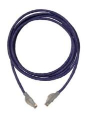
Clarity 6 Modular Patch Cord, purple, 20', Category 6, four-pair UTP stranded 24 AWG PVC/CM, center tuned with Clarity 6 connecting hardware for optimum Category 6 installed performance using Ortronics Paralign 2 pair-positioning technology
