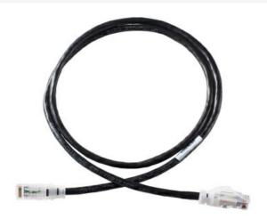
Clarity 6 Modular Patch Cord, black, 25', Category 6, four-pair UTP stranded 24 AWG PVC/CM, center tuned with Clarity 6 connecting hardware for optimum Category 6 installed performance using Ortronics "Paralign 2" pair-positioning technology
