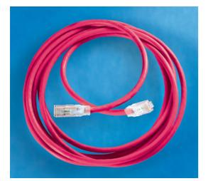
Clarity 6 Modular Patch Cord, red, 15', Category 6, four-pair UTP stranded 24 AWG PVC/CM, center tuned with Clarity 6 connecting hardware for optimum Category 6 installed performance using Ortronics Paralign 2 pair-positioning technology
