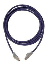
Clarity 6 Modular Patch Cord, purple, 25', Category 6, four-pair UTP stranded 24 AWG PVC/CM, center tuned with Clarity 6 connecting hardware for optimum Category 6 installed performance using Ortronics ''Paralign 2'' pair-positioning technology
