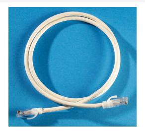
Clarity 6 Modular Patch Cord, white, 25', Category 6, four-pair UTP stranded 24 AWG PVC/CM, center tuned with Clarity 6 connecting hardware for optimum Category 6 installed performance using Ortronics "Paralign 2" pair-positioning technology
