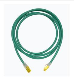
Clarity 6A modular patch cord, green, 3', Cat6A, 10 Gigabit, four-pair UTP stranded 26 AWG PVC/CM, center tuned with Clarity connecting hardware for optimum installed performance using Ortronics Paralign 2 pair-positioning technology.
