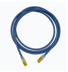
Clarity 6A modular patch cord, blue, 5', Cat6A, 10 Gigabit, four-pair UTP stranded 26 AWG PVC/CM, center tuned with Clarity connecting hardware for optimum installed performance using Ortronics Paralign 2 pair-positioning technology.
