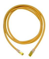
Clarity 6A modular patch cord, yellow, 15', Cat6A, 10 Gigabit, four-pair UTP stranded 26 AWG PVC/CM, center tuned with Clarity connecting hardware for optimum installed performance using Ortronics Paralign 2 pair-positioning technology.
