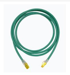
Clarity 6A modular patch cord, green, 15', Cat6A, 10 Gigabit, four-pair UTP stranded 26 AWG PVC/CM, center tuned with Clarity connecting hardware for optimum installed performance using Ortronics Paralign 2 pair-positioning technology.
