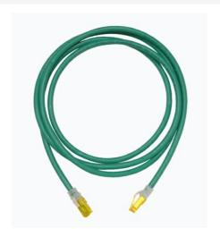
Clarity 6A modular patch cord, green, 25', Cat6A, 10 Gigabit, four-pair UTP stranded 26 AWG PVC/CM, center tuned with Clarity connecting hardware for optimum installed performance using Ortronics Paralign 2 pair-positioning technology.
