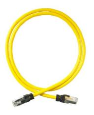
Clarity 6A FTP Modular Patch Cord, yellow, 3', Category 6A, four-pair FTP stranded 26 AWG PVC/CM, center tuned with Clarity 6 A connecting hardware for optimum Category 6A installed performance using Shielded Paralign 2 pair-positioning technology.
