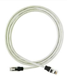
Clarity 6A FTP Modular Patch Cord, gray, 3', Category 6A, four-pair FTP stranded 26 AWG PVC/CM, center tuned with Clarity 6 A connecting hardware for optimum Category 6A installed performance using Shielded Paralign 2 pair-positioning technology.
