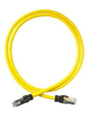
Clarity 6A FTP Modular Patch Cord, yellow, 7', Category 6A, four-pair FTP stranded 26 AWG PVC/CM, center tuned with Clarity 6 A connecting hardware for optimum Category 6A installed performance using Shielded Paralign 2 pair-positioning technology.
