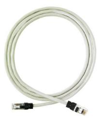
Clarity 6A FTP Modular Patch Cord, gray, 7', Category 6A, four-pair FTP stranded 26 AWG PVC/CM, center tuned with Clarity 6 A connecting hardware for optimum Category 6A installed performance using Shielded Paralign 2 pair-positioning technology.
