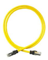
Clarity 6A FTP Modular Patch Cord, yellow, 9', Category 6A, four-pair FTP stranded 26 AWG PVC/CM, center tuned with Clarity 6 A connecting hardware for optimum Category 6A installed performance using Shielded Paralign 2 pair-positioning technology.
