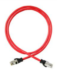
Clarity 6A FTP Modular Patch Cord, red, 15', Category 6A, four-pair FTP stranded 26 AWG PVC/CM, center tuned with Clarity 6 A connecting hardware for optimum Category 6A installed performance using Shielded Paralign 2 pair-positioning technology.
