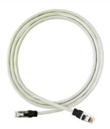
Clarity 6A FTP Modular Patch Cord, gray, 15', Category 6A, four-pair FTP stranded 26 AWG PVC/CM, center tuned with Clarity 6 A connecting hardware for optimum Category 6A installed performance using Shielded Paralign 2 pair-positioning technology.
