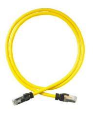
Clarity 6A FTP Modular Patch Cord, yellow, 20', Category 6A, fourpair FTP stranded 26 AWG PVC/CM, center tuned with Clarity 6 A connecting hardware for optimum Category 6A installed performance using Shielded Paralign 2 pair-positioning technology.
