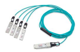
4m Mellanox/NVIDIA MFA7A50-C004 Compatible 100GBase-AOC QSFP28 to 4 x SFP28 Breakout (MMF, 850nm, LSZH) Active Optical Cable
