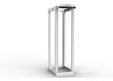
Mighty Mo 20 Dual Adjustable Base 4-post racks provide greater flexibility and optimum efficiency in any data center or telecom room. The base angles adjust in depth with the rails reducing the overall footprint when the rail spacing is reduced. Front and rear waterfalls allow for equipment patching and server patching. All styles of Mighty Mo 20 vertical managers can be mounted to the front or rear.
