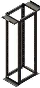
Mighty Mo 20 4-post racks fixed racks provide an economical mounting platform for switches and servers. Front and rear waterfalls allow for equipment patching and server patching. All styles of Mighty Mo 20 vertical managers can be mounted front or rear and airflow baffles can be mounted to manage the airflow of side breathing equipment.
