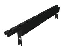
$Mounts\ to\ the\ top\ side\ of\ the\ Mighty\ Mo\ rack\ channels\ or\ frames\ and\ provides\ tool-less\ mounting\ for\ Cablofil\ cable$ tray to run parallel with the row of racks. Standard brackets position the bottom of the tray at 2" above the rack height and 6" high brackets position the bottom of the tray at 6" above the rack height.
