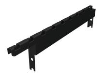
$Mounts \ to \ the \ top \ side \ of \ the \ Mighty \ Mo \ rack \ channels \ or \ frames \ and \ provides \ tool-less \ mounting \ for \ Cablo fill \ cable$ tray to run parallel with the row of racks. Standard brackets position the bottom of the tray at 2" above the rack height and 6" high brackets position the bottom of the tray at 6" above the rack height.
