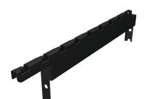
$Mounts \ to \ the \ top \ side \ of \ the \ Mighty \ Mo \ rack \ channels \ or \ frames \ and \ provides \ tool-less \ mounting \ for \ Cablo fil \ cable$ tray to run parallel with the row of racks. Standard brackets position the bottom of the tray at 2" above the rack height and 6" high brackets position the bottom of the tray at 6" above the rack height.
