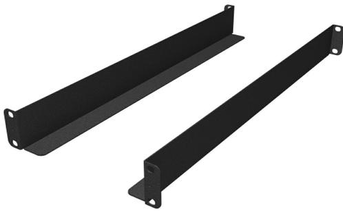
The 6" equipment support brackets can be cantilever mounted at the rear of any Mighty Mo rack and used to support equipment mounted to the front rails. Deeper equipment support brackets are sized to the 16-1/4" to 30" channel racks and 4-point mount with the equipment's mounting ears to provide zero unit support from front to back.
