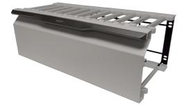
Horizontal cable managers are available in 2RU and 4RU sizes. Fingers begin 3/4 in from the face of rack to provide bend limitation for cables, protecting cables, equipment and network performance. Included hinged cover mounts with six heavy duty clips allow them to be
