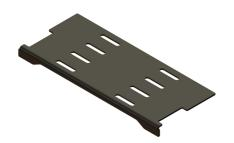
Zero rack unit horizontal managers slide into the slots in the Mighty Mo 20 fingers and provide support for fiber and copper cables exiting horizontal equipment modules. They toollessly lock into place with the 19" version mounting between 2 vertical managers in front of the equipment. Internal versions are sized to fit inside the vertical managers and provide a continuous horizontal path across the front of the racks and managers.
