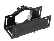
Universal cable troughs snap into the hex pattern on the Mighty Mo 20 channel racks and are used to create a front to rear or vertical trough on the inside or outside of the channel. They can be mounted in a row to create a continuous trough or rotated at 30 degree increments to support cables through directional changes. Up to 3 HiLOC harnesses can be toollessly mounted into each trough. The 2" x 2" size is equipped with slots to allow it to be joined to Mighty Mo Fiber Raceway.
