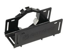
Universal cable troughs snap into the hex pattern on the Mighty Mo 20 channel racks and are used to create a front to rear or vertical trough on the inside or outside of the channel. They can be mounted in a row to create a continuous trough or rotated at 30 degree increments to support cables through directional changes. Up to 3 HiLOC harnesses can be toollessly mounted into each trough. The 2" x 2" size is equipped with slots to allow it to be joined to Mighty Mo Fiber Raceway.
