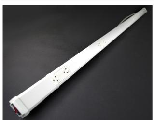
Ten (5 duplex) outlets, nonmetallic housing with ivory finish. 6' (1.8m) cord. Length 48'' (1.2m). Receptacle center-to-center 12'' (305mm).
