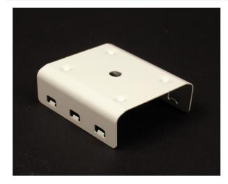
Support lengths of raceway at any point desired. Mount to surface with No. 8 flathead screw.
