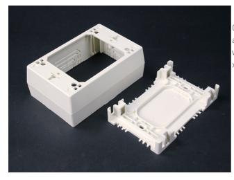
Cover snaps onto base - no screws required. Cover has twistouts on all sides. Rectangular KO in base for extensiion to wall box. Used with 2700, 2800, 2900 and NM2000 Series Raceways. 4 3/4'' L x 3'' W x 1 3/4'' D (121mm L x 76mm W x 44mm D). 1-Gang.
