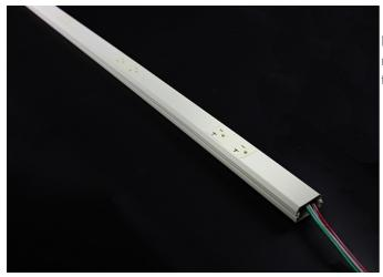
Nonmetallic Plugmold with alternating circuits. 6' in length with receptacles spaced 12'' on center. Nonmetallic plugmold has a textured finish ivory finish, For use with 20 amp circuits.
