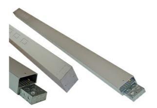
Two-compartment large capacity pole. Furnished unwired without outlets. Box ended with industry sized knockouts. Standard heights: 10' 2" (3.1m) (NP800C-10-2B), 12' 8" 3.9m) (NP800C-12-8B), 15' 2" (4.6m) (NP800C-15-2B)
