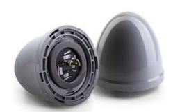
The NWTL-111 BULIT is a distributed-intelligence wireless control node designed to replace standard photocell modules on outdoor lighting fixtures. It connects to a 7-pin twist-lock receptacle compliant with NEMA standard C136.41 to provide ON/OFF and dimming control. The BULIT also connects to a Legrand Wireless Network Manager via a robust and scalable self-healing wireless IP network.
