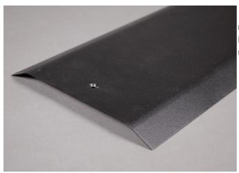
Cover: 0.040" (1.0mm) steel. Durable black powder coat finish. Packed four (4) 8' (2.4m) lengths of cover per carton. NOTE: Not recommended for use in high traffic areas.
