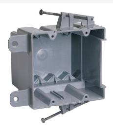
Two-Gang Switch and Outlet Box with captive mounting nails on each end and threaded mounting holes. It has four Auto/Clamps on each end. It is made with durable, impact-resistant thermoplastic. It is easy to install with a rectangular cutout. 100 pack.
