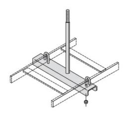
Cable Runway is available with tubular side rails that are lightweight yet strong and utilize rungs are made of tubular steel. Powdercoated finish is available in standard black.
