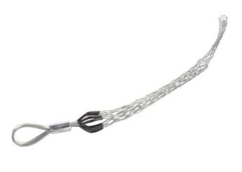
Multi-Weave, Rotating Eye. Cable Diameter - 3.000-3.490-inch, Mesh Length - 54-inch, Eye Diameter - 1 7/8-inch, Break Strength - 48,000 lbs, Aluminum.
