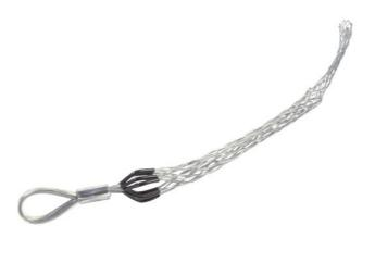
Multi-Weave, Rotating Eye. Cable Diameter - 3.500-3.990-inch, Mesh Length - 56-inch, Eye Diameter - 1 7/8-inch, Break Strength - 48,000 lbs, Light Green.
