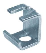
Use open clips with 1-1/2 in stringers to secure runway to threaded rods when suspending runway from the ceiling. Also use when stacking runway. Use with 5/8 in-11 in threaded rod. Made of 3/16 in x 1-1/2 in steel bar. UL classified.
