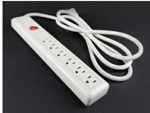
P6 includes six outlets in a putty white impact-resistant housing. Delivers 15A of power with a lighted switch. Includes 6ft 14/3 SJT white cordwith NEMA 5-15 plug.
