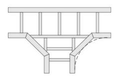
For extremely corrosive applications we offer a full line of straight sections, fittings, covers and mounting accessories in polyester and vinylester fiberglass. Rail heights are available in 4" and 6" and widths are available up to 36".
