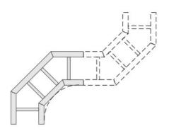
Choose from an extensive selection of metallic ladder tray with a variety of rung and bottom styles to choose from. Finishes include steel, 304L and 316L stainless steel to meet the needs of any application. Rail heights range from 4" to 7" and width sizes are available up to 36".
