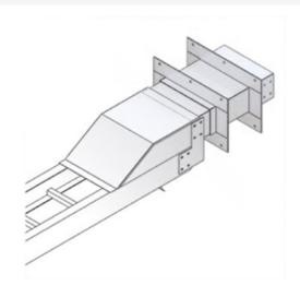
Choose from an extensive selection of metallic ladder tray with a variety of rung and bottom styles to choose from. Finishes include steel, 304L and 316L stainless steel to meet the needs of any application. Rail heights range from 4" to 7" and width sizes are available up to 36".
