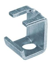
Use open clips with 1-1/2 in stringers to secure runway to threaded rods when suspending runway from the ceiling. Also use when stacking runway. Use with 5/8 in-11 in threaded rod. Made of 3/16 in x 1-1/2 in steel bar. UL classified.
