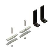
Cable runway feet anchor runway to the wall or floor. Feet are attached to runway with clamps. Made of 3/8 in x 1-.5 in, steel bar. Kit includes two 6 in. cable feet, four straight clamps, two 3/8-16 x 2.25 in carriage bolt, and two 3/8-16 hex nut.
